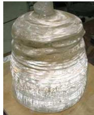
The installations used for sapphire growth, have been developed by Ukrainian scientists. They are capable to produce sapphire crystals from the sintered aluminum oxide by Kiropulos method, weighing from 35 to 85 kg. This installation has is the **best installation for sapphire crystal growing among the parallels.**
